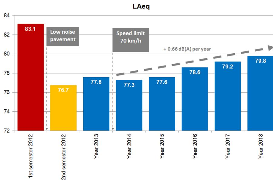
Figure 3 – Evolution of the average noise level LAeq calculated per year since 2012.
