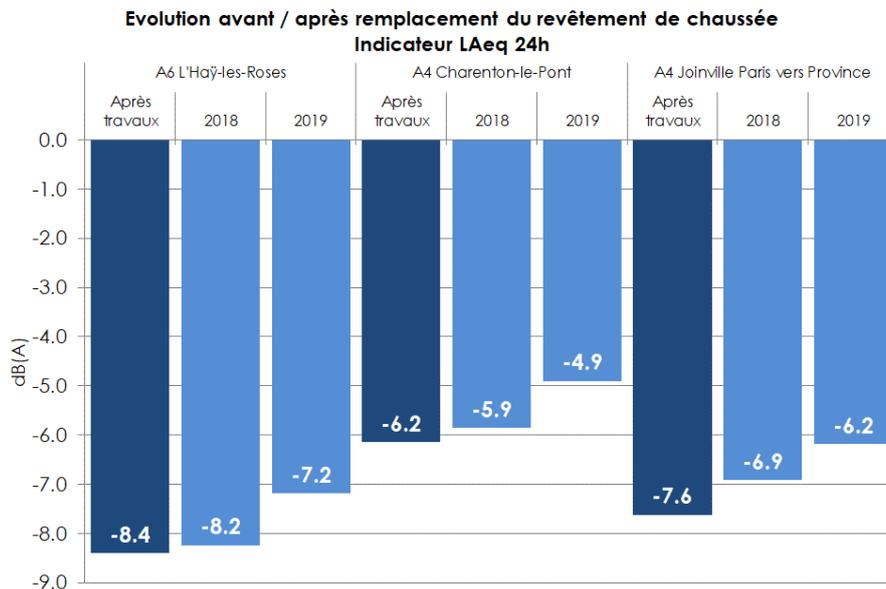
Figure 5 – Evolution before / after road surface replacement; LAeq indicator 24h.
