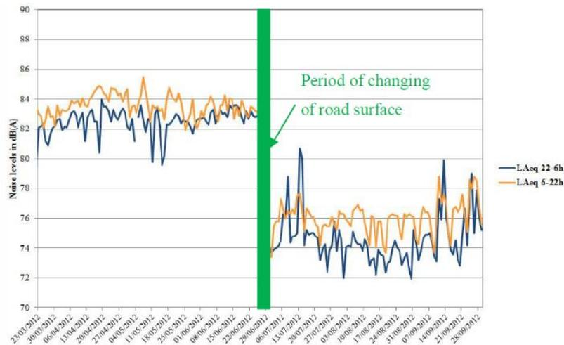
Figure 1 – Reduction of day and night noise levels near the source (median) after the pavement change.
