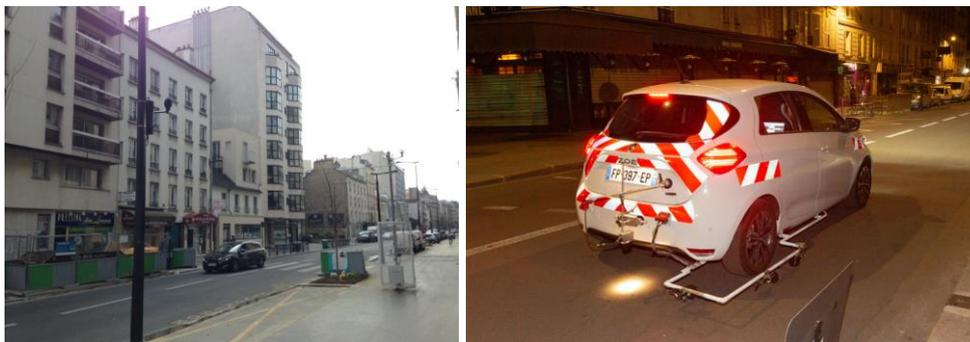
Figure 7 – Acoustic station and thermal station; CPX measuring equipment (City of Paris); Frémicourt street 75015 Paris (SMaphon).
